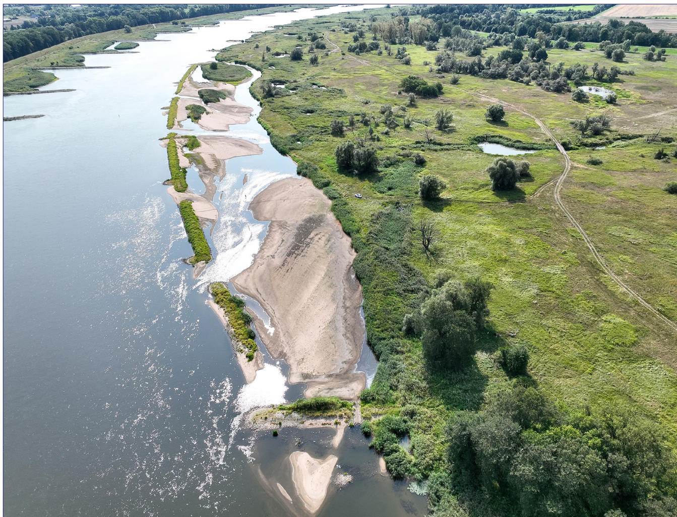
Fig. 1: Longitudinal training wall (LTW) in the Oder River near Reitwein. Aerial image looking upstream taken by the WSA Oder-Havel on 23 August 2024 with different currents and diverse habitats in the secondary channel ( W = 141 \text{ cm} [ +8 \text{ cm} to MLW]) at reference gauge Frankfurt1 (Oder), 23 August 2024 09:30)
